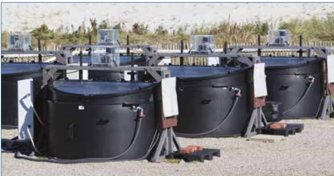
Figure 3: Sylt Mesocosms: Effects of climate change (i.e. increased temperature, CO 2 and nutrient concentrations) on intertidal communities of the Wadden Sea were tested in 12 tanks each holding 1800 l of seawater. Currents and tidal conditions were also simulated.
