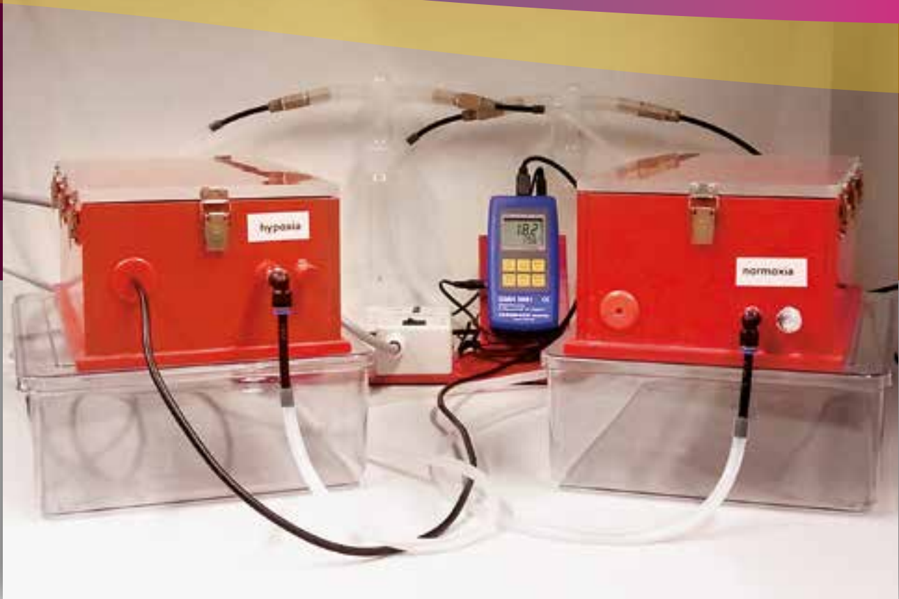
Figure 2: One of the signaling pathways being researched in the Sybacol consortium is the hypoxia signaling pathway. To generate conclusive findings, the worms must be subjected to a precisely defined level of hypoxia (oxygen deprivation) for a certain period of time. As no suitable equipment is available for this, special hypoxia chambers were developed and constructed in close collaboration with research scientists and workshops at the University Hospital (Source: Martin Höhne).
