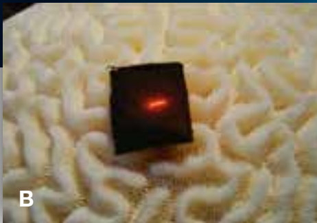
Figure 2: A + B Multiple scattering by a coral skeleton. Comparison of light scattering patterns from a laser pointer directed in A at a coral skeleton, with the same laser beam in B reaching an opaque plastic target. C Naturally bleached Orbicella faveolata colony in the Caribbean (Photos: R. Iglesias-Prieto).
