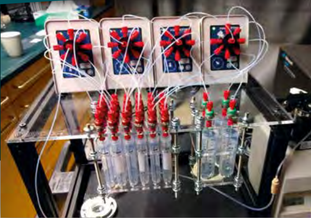
Figure 3: The flow system constructed by Jeffrey Moffitt. Each tube contains a different stain that we will apply to our sample. The system is completely computer controlled and automated, so each of these stains will be flown across the sample at the appropriate time (Source: Jeffrey Moffitt).
