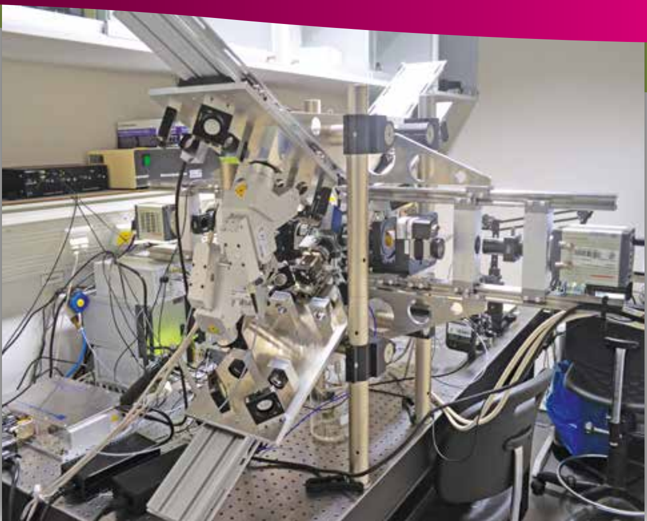
The X-Wing is a microscope that is used to record images of and track all cells in a developing Drosophila embryo. The microscope gets its nickname from its four arms, which project laser beams into the embryo, and make the microscope look like an X-wing spaceship from Star Wars . The two other arms at the front and back each contain a very high-resolution lens and a specially controlled camera. In total, six lenses and a lot of control software developed in-house are used in order to achieve the highest possible image quality without affecting the development of the organism being observed (Photo: M. Colindres).
